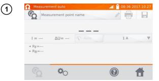
The measurement is performed as in the case of testing the inductive objects If based on the difference between the instantaneous and average resistance during the result stabilization, the meter determines that the object is resistive, it will complete the measurement faster.
